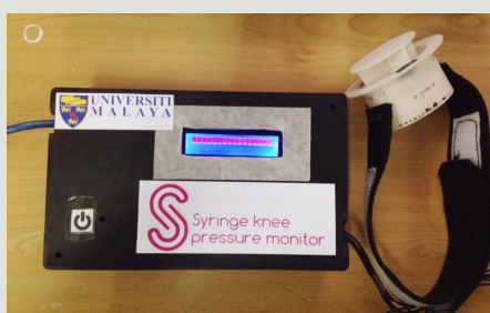
Photo 2: Syringe Knee Pressure Monitor
